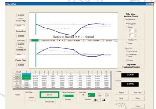
Bore8 Software showing plot of bore straightness.
