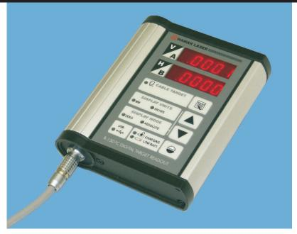
The R-1307C, shown above, replaces Hamar Laser's R-307 Analog Readout and supports local (cabled) targets.
